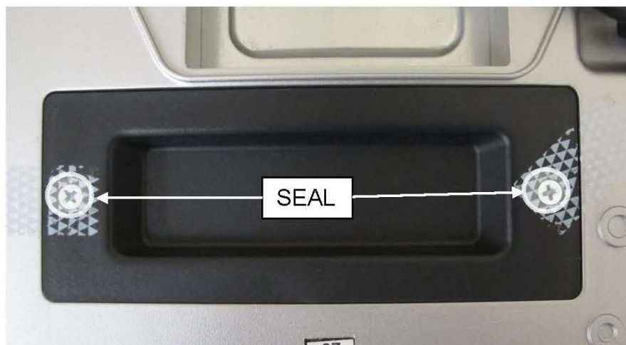
(a) Typical Sealing Arrangement – Bench Style Instruments
