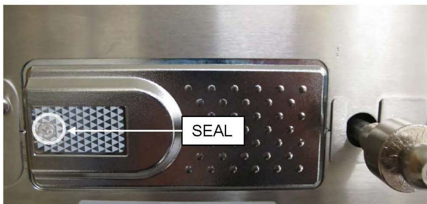
(b) Typical Sealing Arrangement – Hanging Style Instruments
