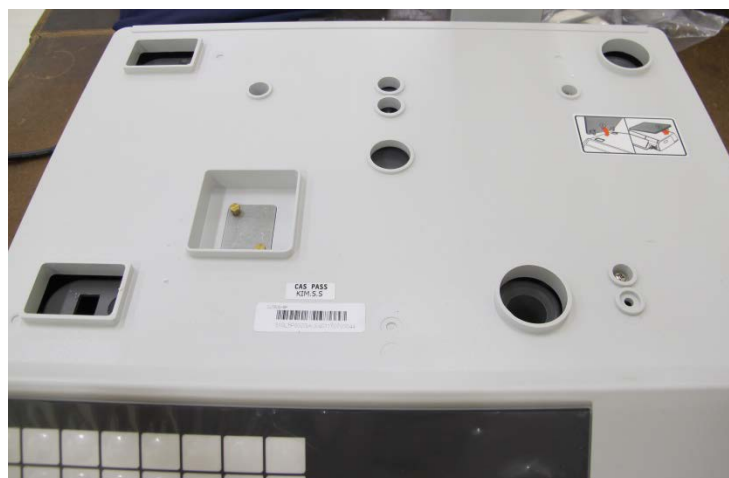
Showing Typical Sealing of the Model CI 5500-6P (Pattern)
