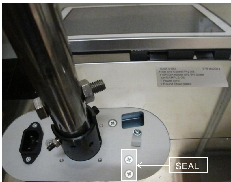
Typical Sealing Arrangements – Model UNI-9 H (variant 7)
