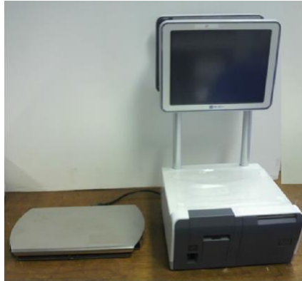
(a) Ishida Model UNI-9 Using a Slim Remote Basework (variant 9)
