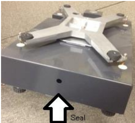
(a) Sealing Arrangements – Model S3-Z60 30 kg Remote Basework (variant 7)
