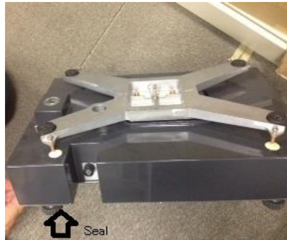
(a) Sealing Arrangements – Model S3-Z60 30 kg Remote Basework (variant 7)
