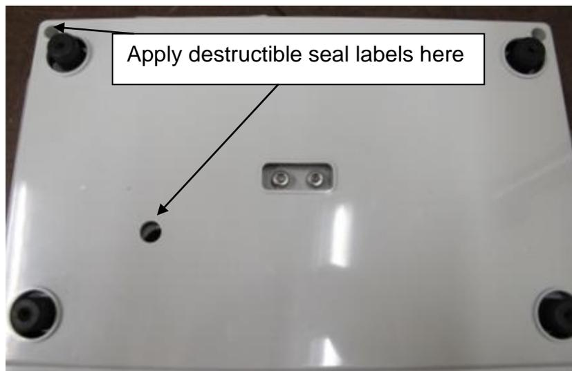
Typical Mechanical Sealing
