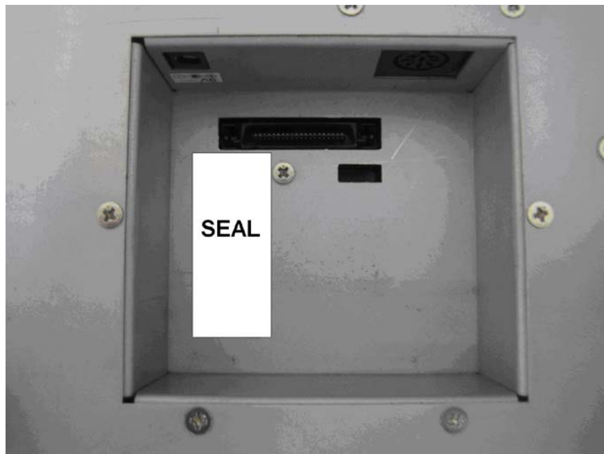
(b) Sealing of calibration access point
