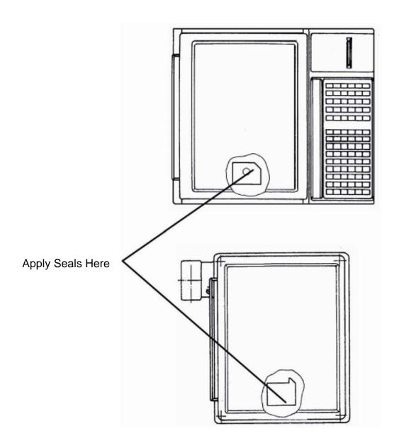
Typical Mechanical Sealing of Bizerba SC II Series
