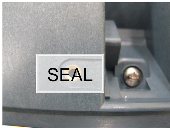
(b) Sealing of Span Switch Access Hole with a Destructible Adhesive Labels
