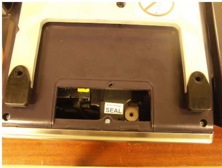
Sealing of Calibration Switch Access Hole and Security Screw (Shown with protective cover removed)
