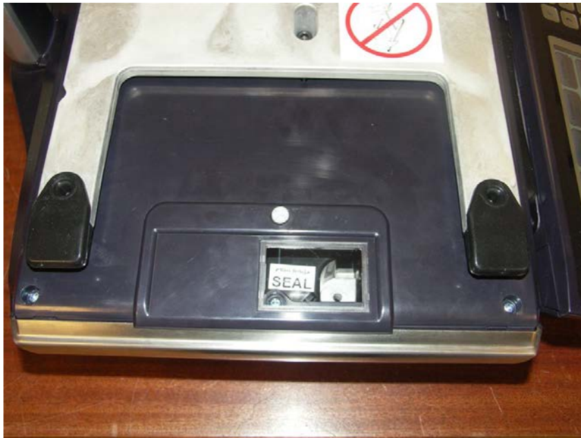
(a) Position of Seal Label - Viewed through Protective Cover
