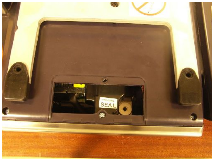
(b) Sealing of Calibration Switch Access Hole and Security Screw (Shown with protective cover removed)
