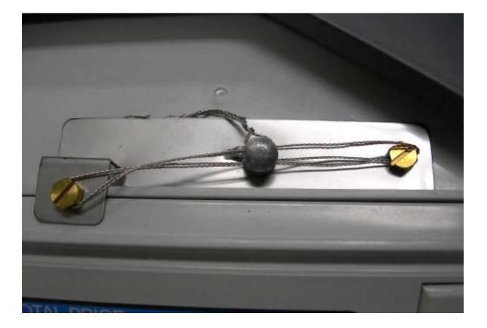
Sealing of Calibration Access Hole – Beneath Instrument
