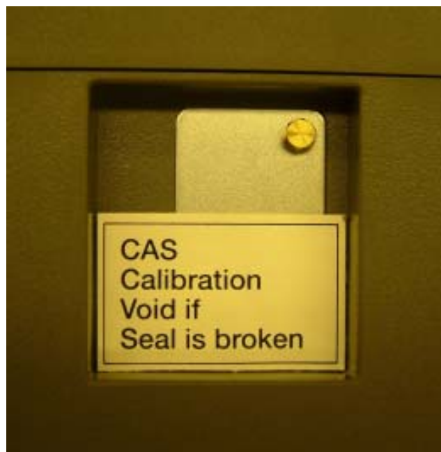
(a) Alternative Sealing of Calibration Access Hole – Beneath Instrument
