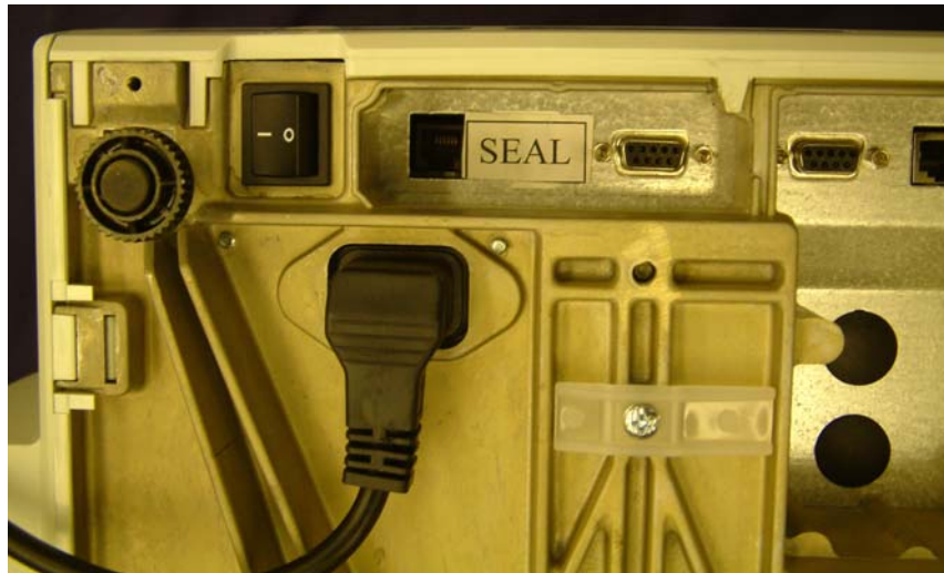
Sealing of Calibration Access Hole – Beneath Instrument
