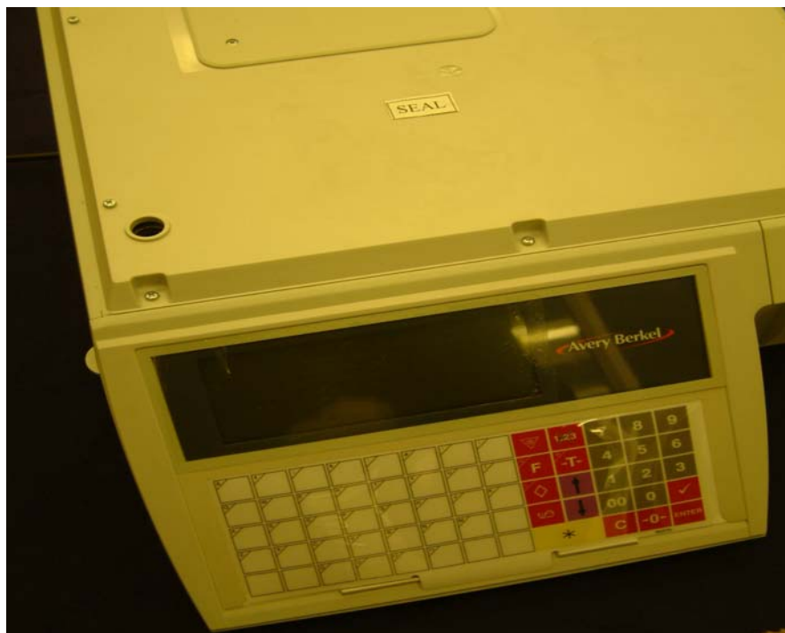
Sealing of Calibration Access
