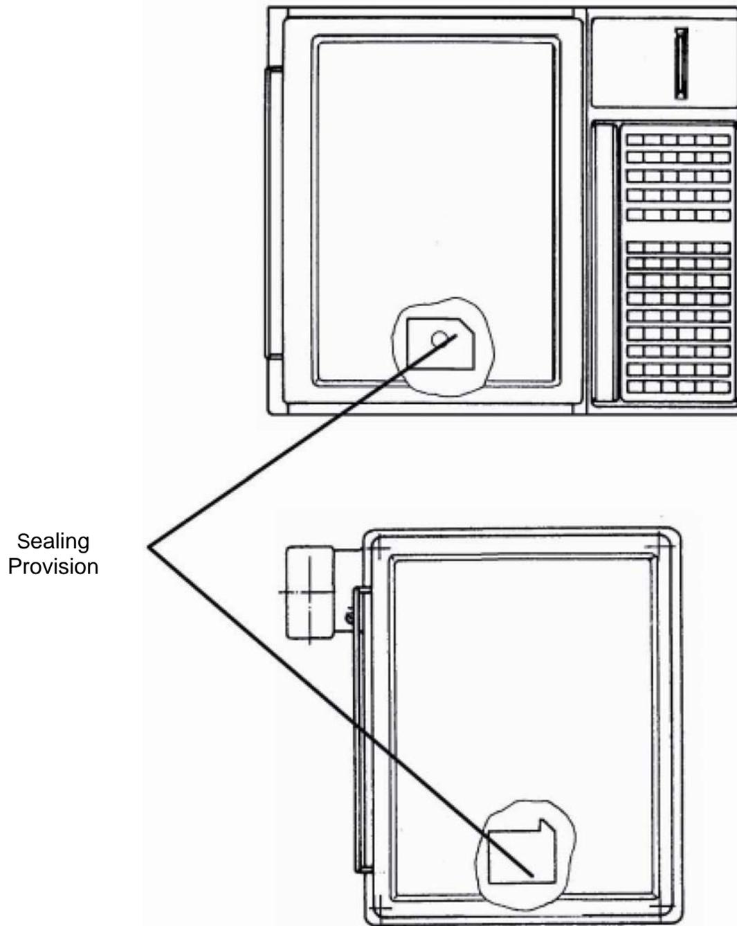
Sealing of Calibration Access
