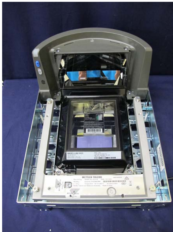
(b) Mettler Toledo Model Ariva-B Weighing Instrument With Load Receptor Plate Removed (Variant 2)
