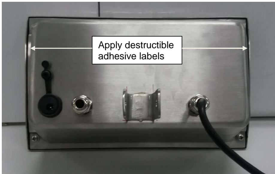
(a) Typical Sealing of Wedderburn Model WDI-702 Stainless Steel Indicator (Pattern & variants)
