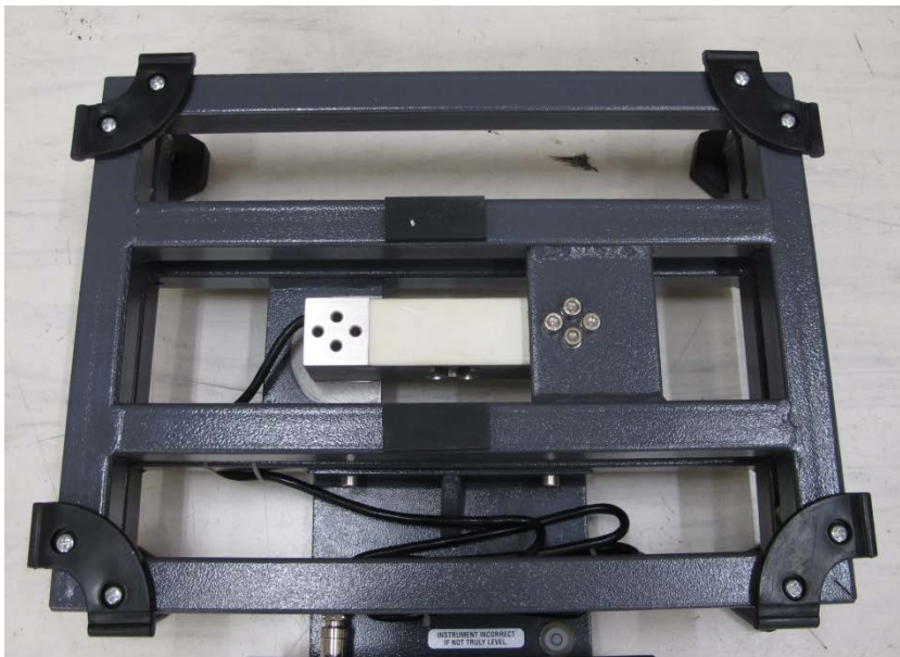
(b) Wedderburn Model TMS Basework Mounting Frame (Variants 6 & 7)
