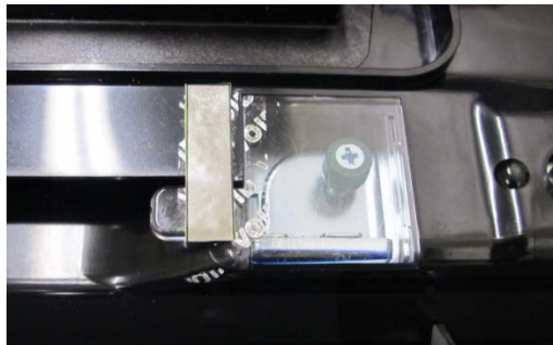
(b) Typical Sealing Using a Destructible Adhesive Label
