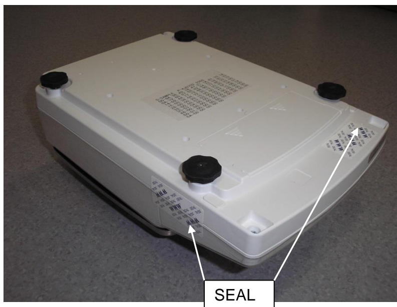
Typical Sealing Arrangement Using Destructible Adhesive Labels
