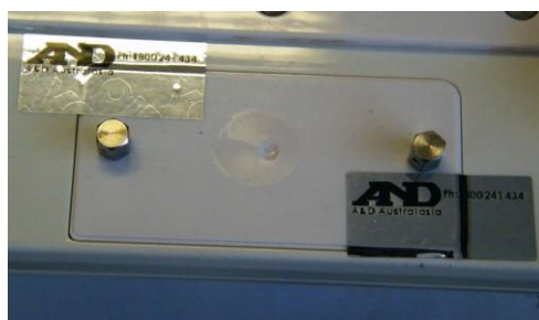
(b) Destructible Adhesive Stickers Sealing Arrangement
