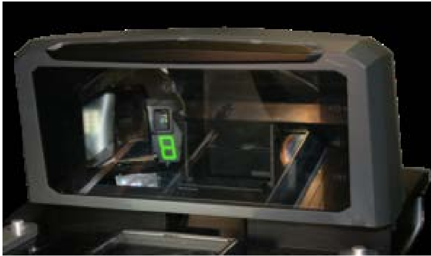
Seven Segment LED Display for Calibration and Configuration Event Counters
