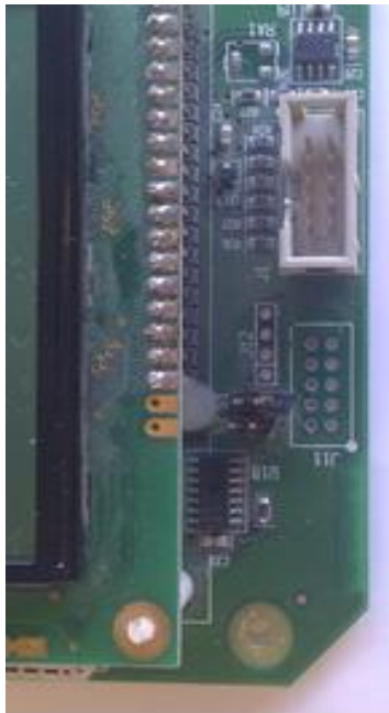
S1 Calibration Jumper
