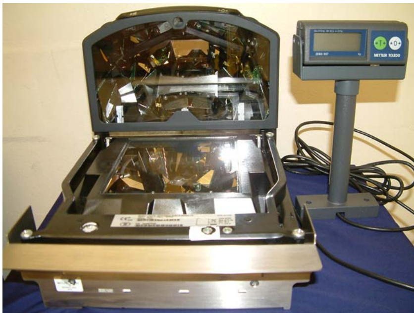
(b) Mettler Toledo Model DIVA Weighing Instrument With Load Receptor Plate Removed
