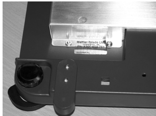
(d) Destructible adhesive label applied to the PCB cover as shown
