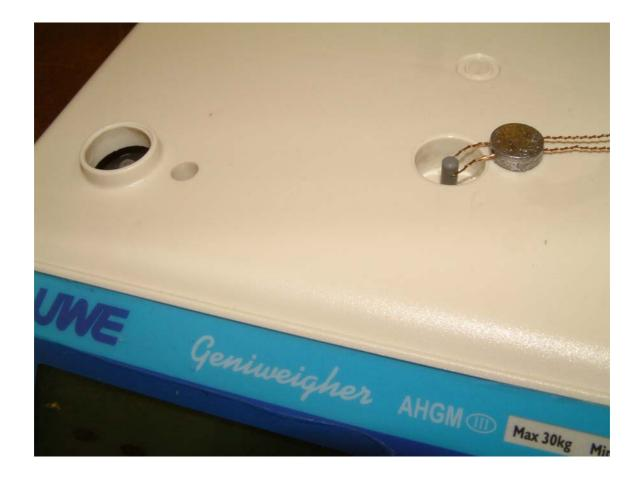
Sealing location beneath platter. Ensure seal does not interfere with the platform.
