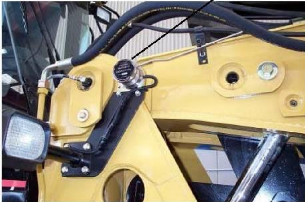
Typical Loadrite Model LR908 Rotary Sensor Installation
