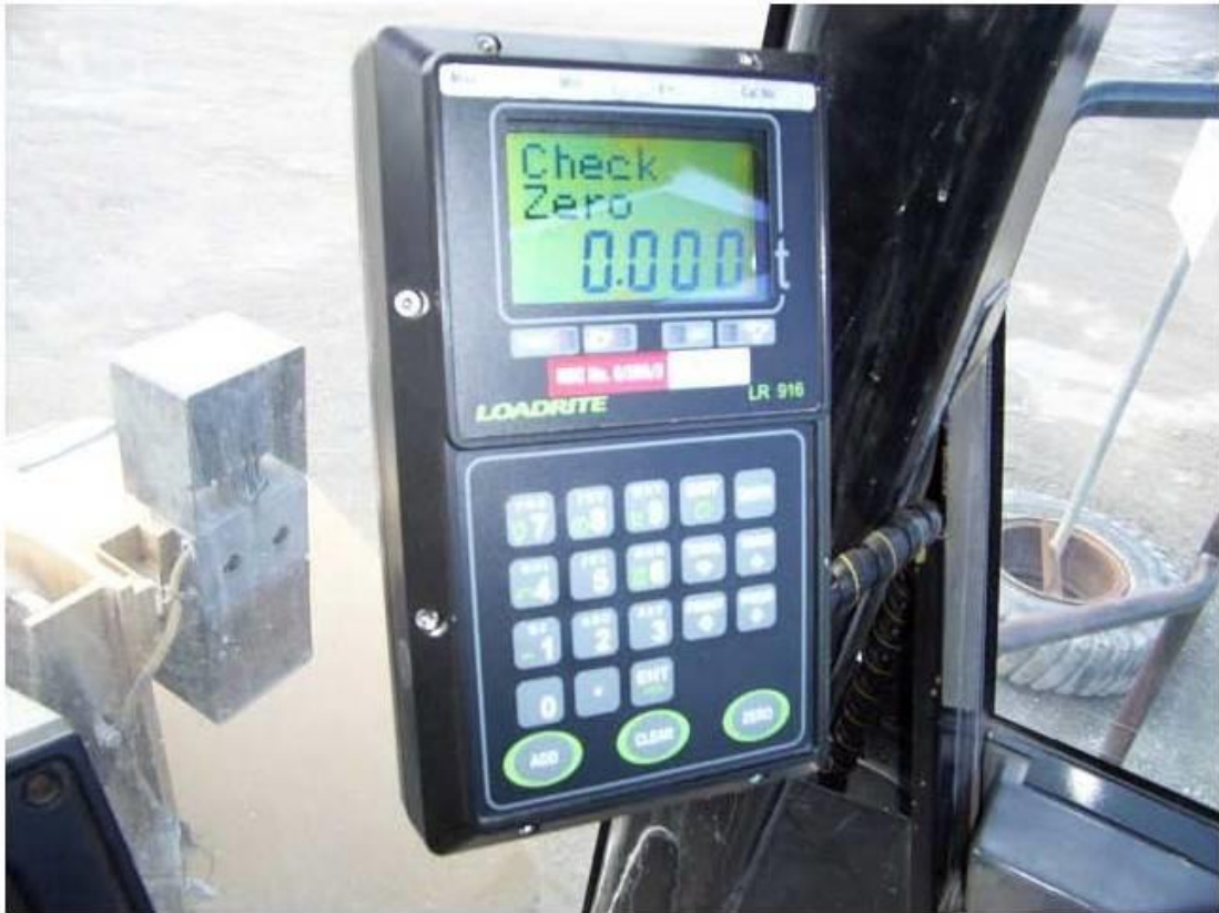
Loadrite Model LR916 Computing, Keyboard and Display Unit (Pattern)
