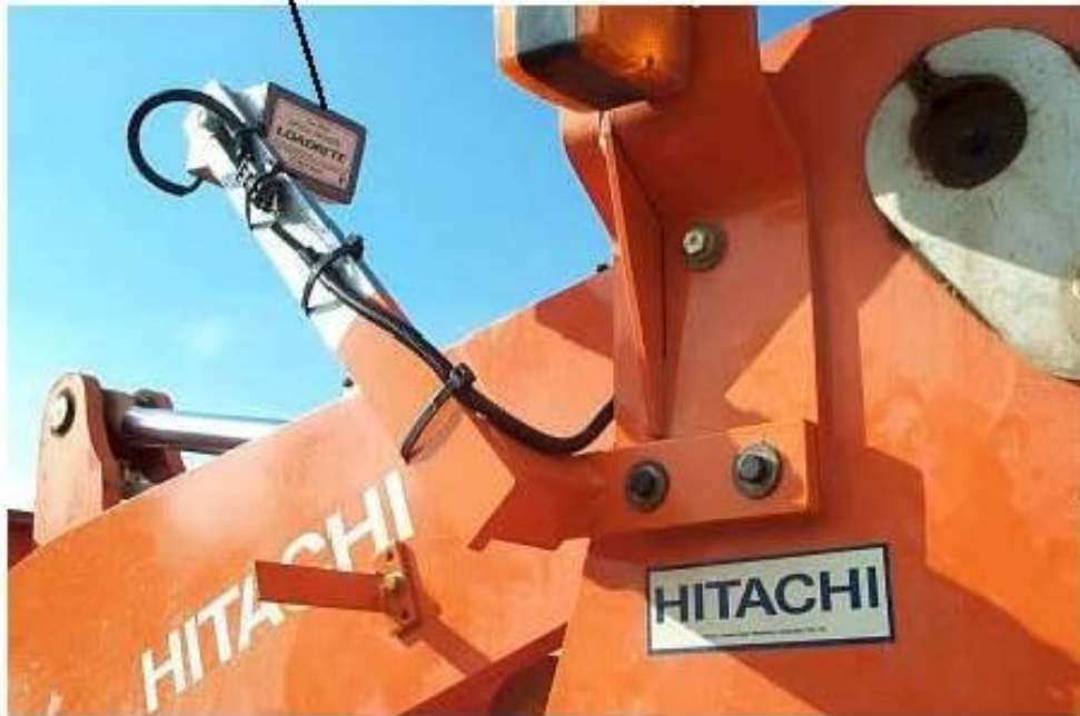
Typical Loadrite Model LM960 Optical Sensor Installation
