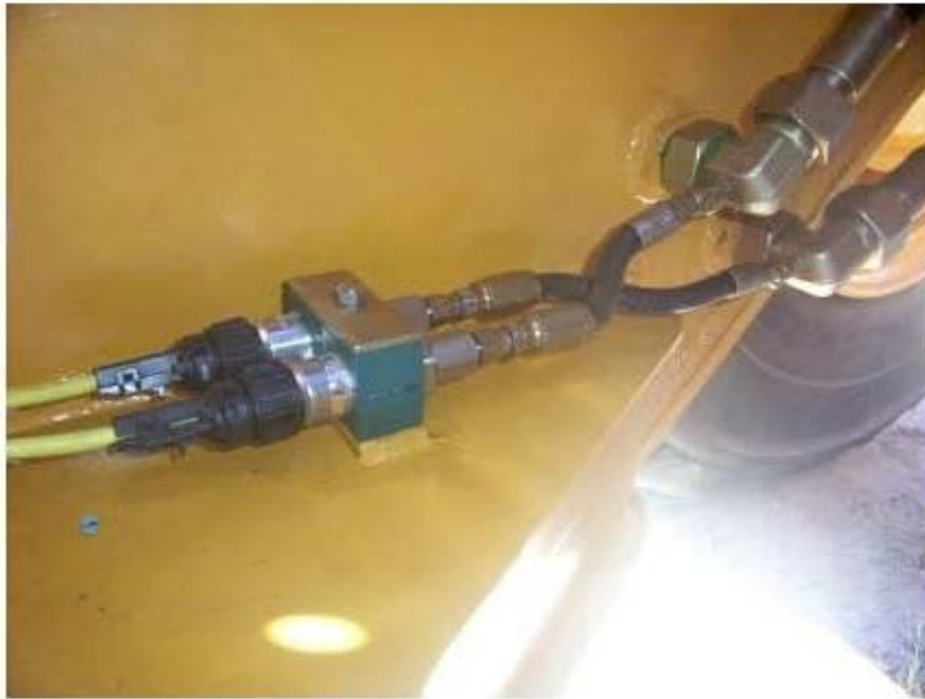
Typical Loadrite Model LC965 Pressure Sensor Installation
