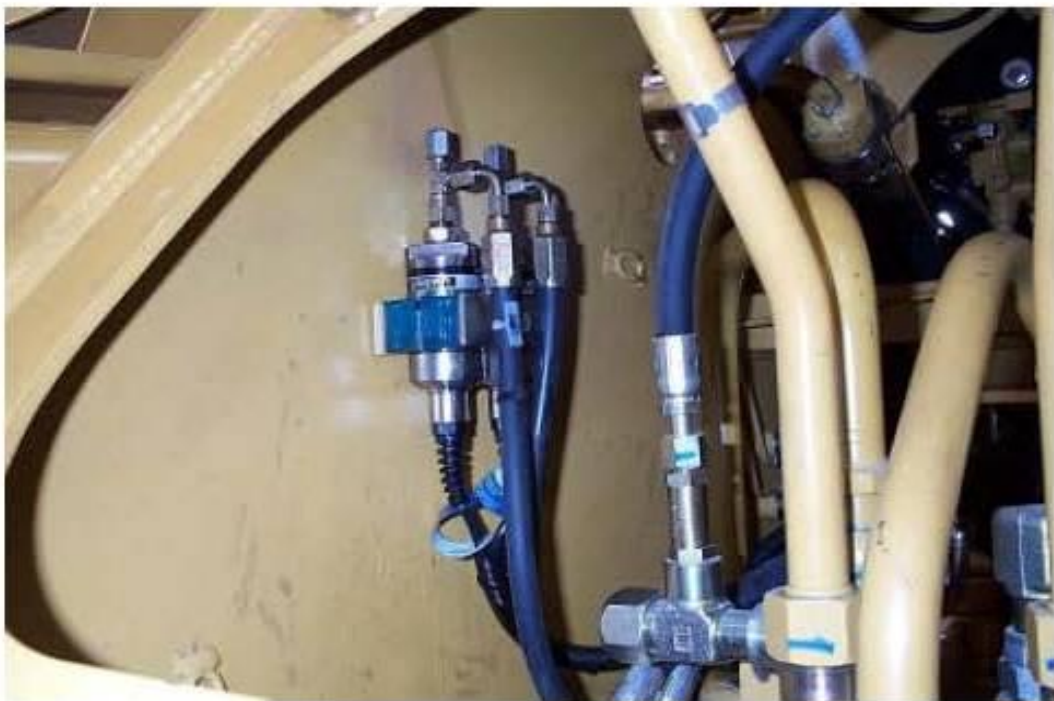
Typical Loadrite Model LC340 Pressure Sensor Installation
