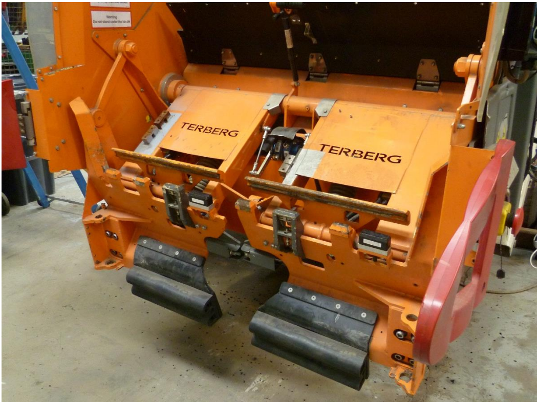
Load Cell (Installed Behind The Load Receiver Frame) AMCS Model VDH Wheeled Loader Weighing Instrument
