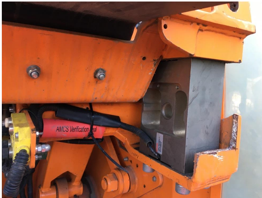
(a) Load Cell (Installed Behind The Load Receiver Frame)
