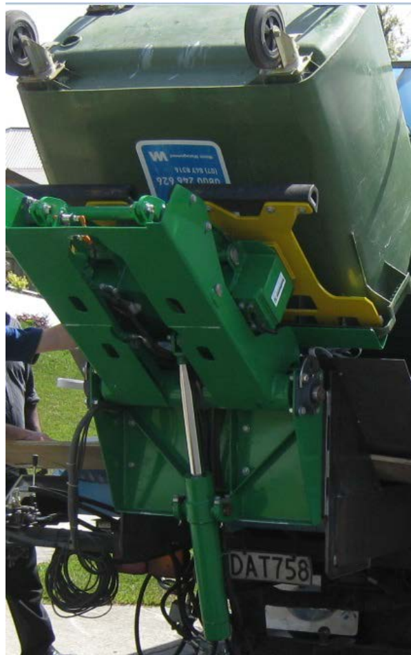
(a) Accuonboard Model Binweigh LFT RL operating in mode weighing single larger bin
