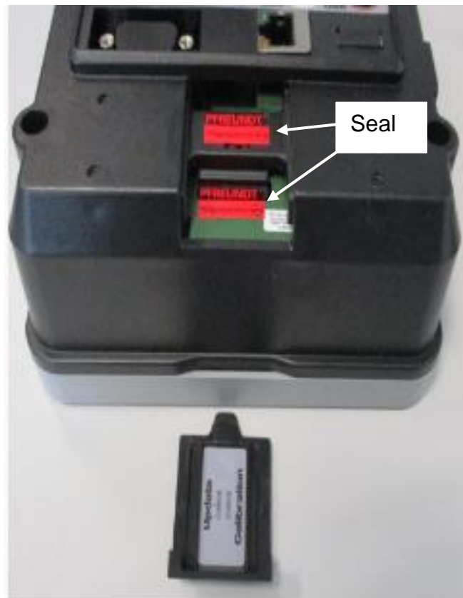
(b) Typical Sealing of WK60 Control and Display Unit
