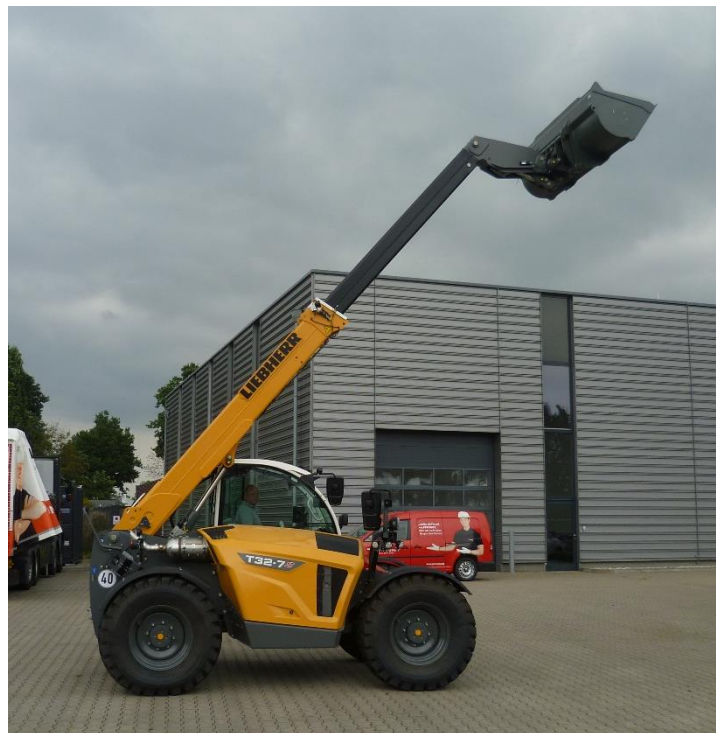
(f) Typical Pfreundt Model WK60 Telescopic Wheeled Loader Weighing Instrument (Variants 3 and 4)
