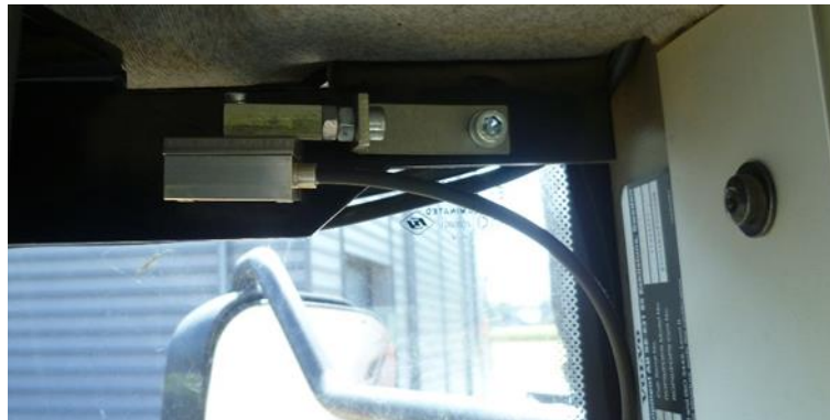
(c) Pfreundt Model LS1 Inclination Sensor
