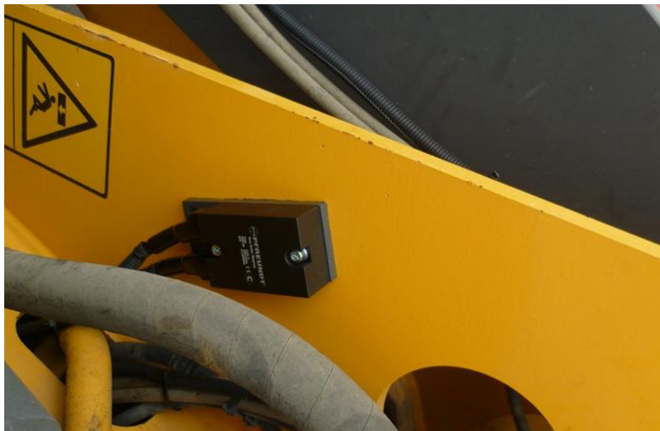
Pfreundt Model CLS1-# Chassis Inclination Sensor
