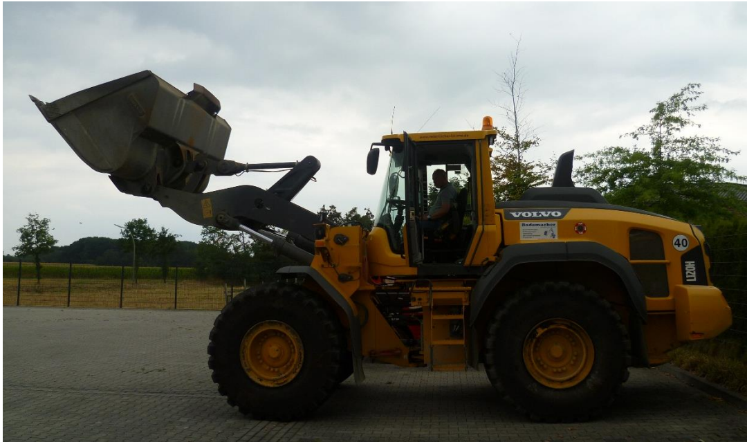
(e) Typical Pfreundt Model WK60 Wheeled Loader Weighing Instrument (Pattern and Variant 1)
