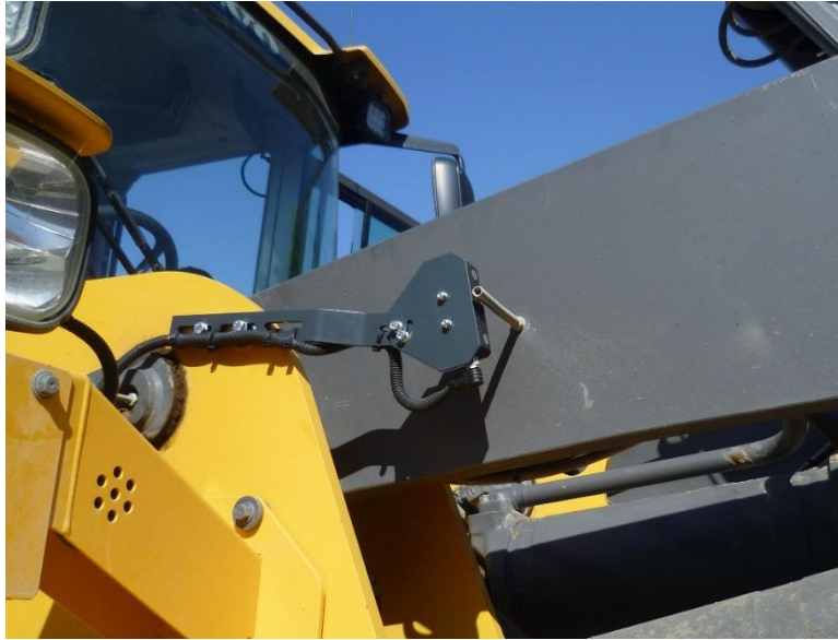
(a) Pfreundt Model N1 Boom Angle Sensor
