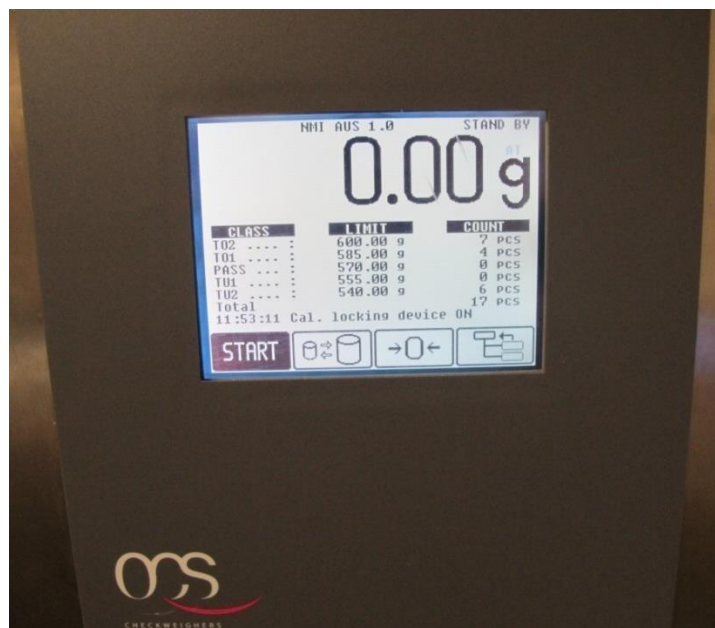
OCS/Wipotec Model RC-TERM Indication Unit (Variants 8 to 12), integrated into a switch cabinet (refer to Figure 9)
