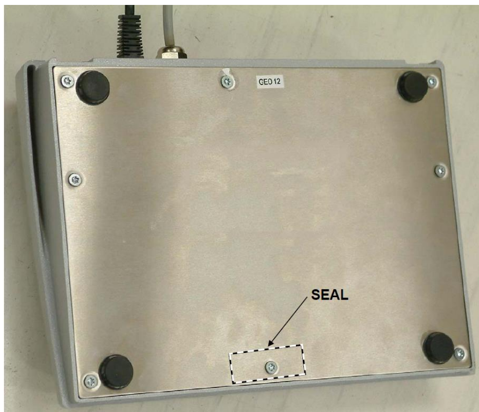
(b) Sealing of IND 439 Control/Indication Unit
