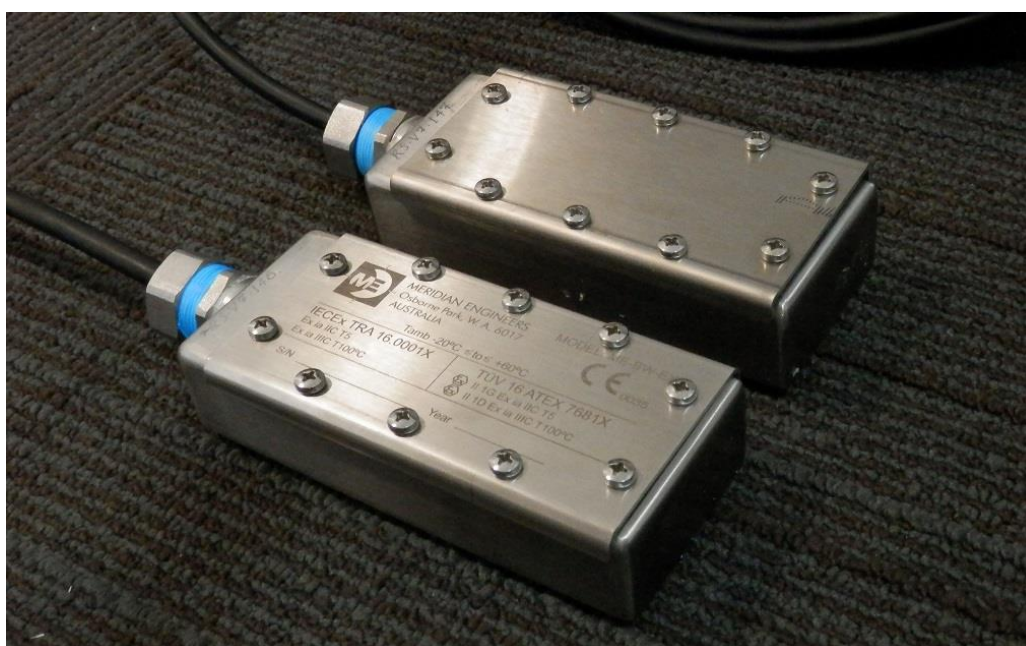
Transducers used in ME-RailType-nB and ME-RailType-nEX 'rail load cells'
