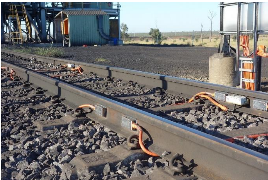
ME-AS60-2B 'rail load cells', showing their location on sleepers and track switch mounting.
