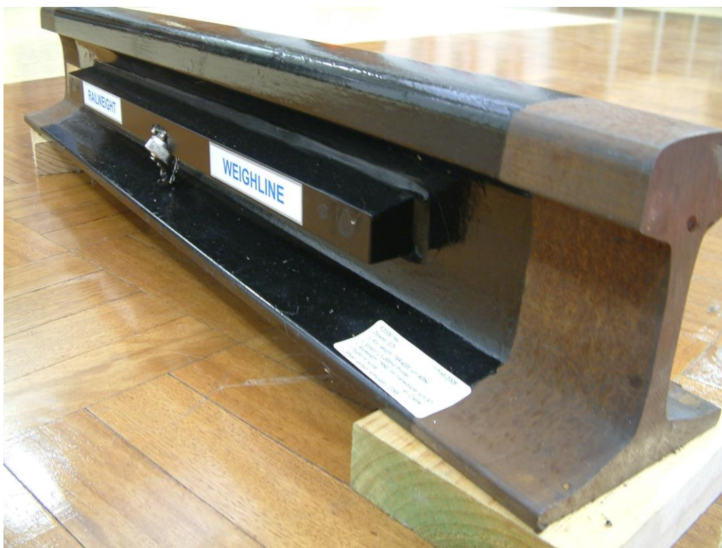
(a) Railweight Model WEIGHLINE RWT-X TR60 Weighing Transducer
