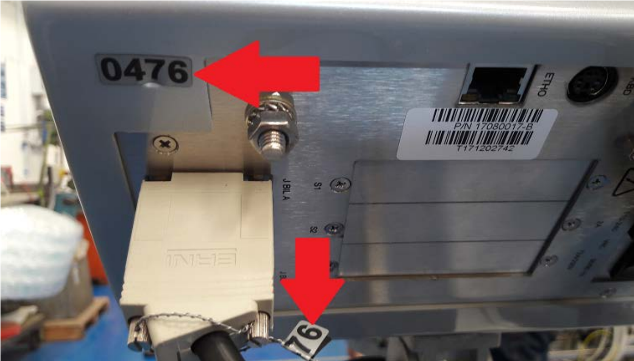
(a) Sealing on calibration switch and load cell cable (seal by applying destructible adhesive label or lead and wire or similar type seals )
