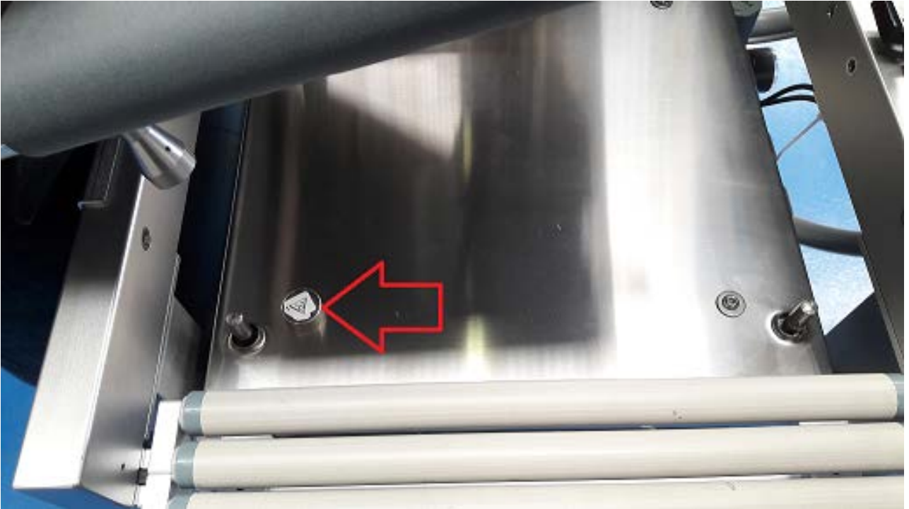
(b) Sealing on screw of load receptor (below the weighing receptor conveyor) to avoid opening of the protective shell
