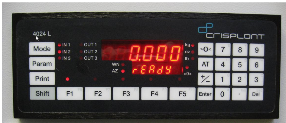
(c) Crisplant Model 4024L Display Module (manufactured by Eilersen Electric)
