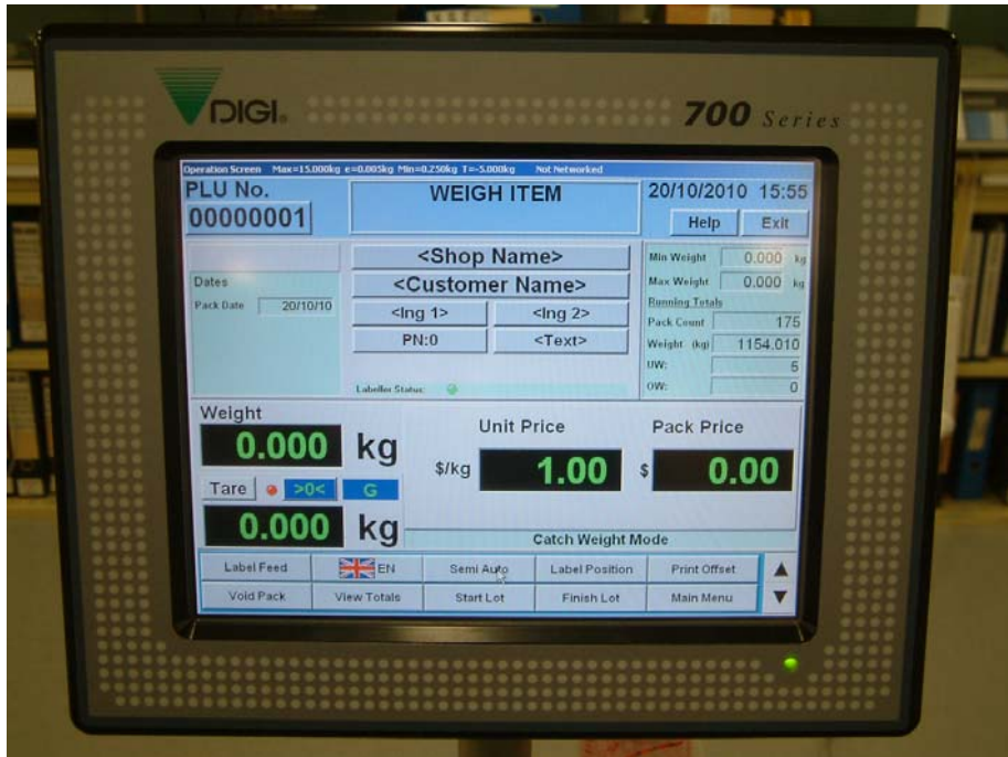
(a) Digi Model 700 Series Terminal/Indicator
