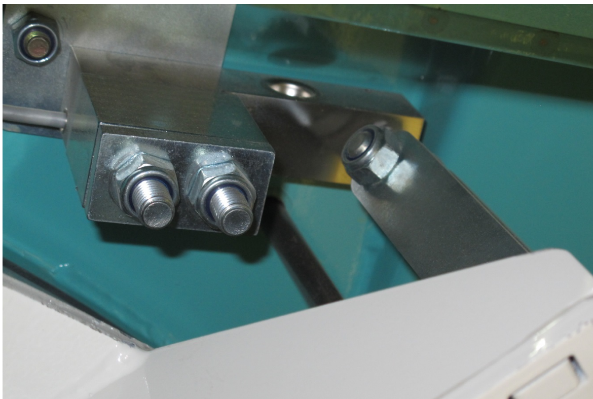
HBM Model HLCB1C3 1.76T load cell, mounting arrangement
