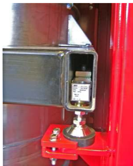
(b) Load Cell Mounting
