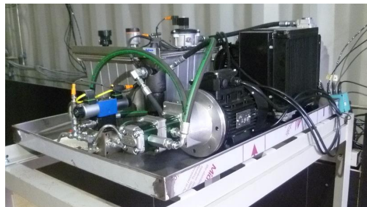
(b) Hydraulic Power Unit
