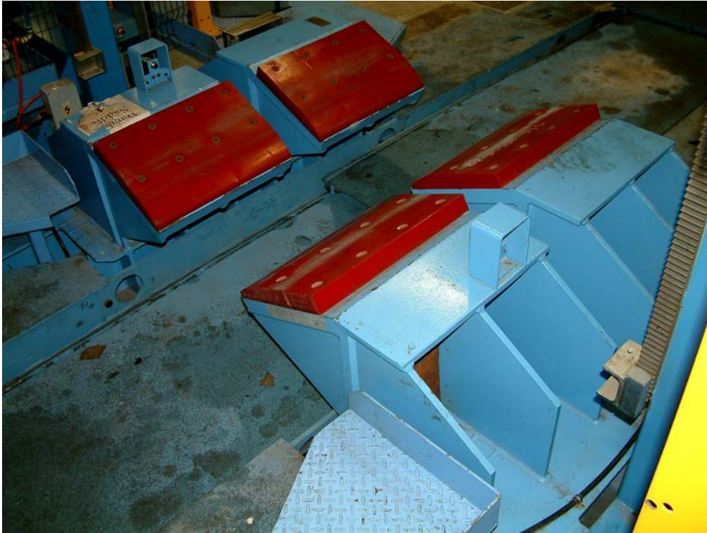
(a) BSS coil weighing instrument basework (coil rests on the (red) pads)
