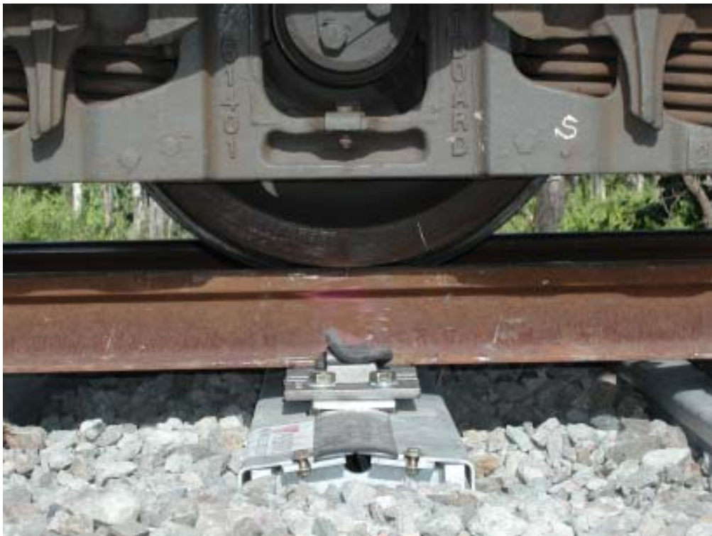
Pfister Model SOLAR Sleeper Module
