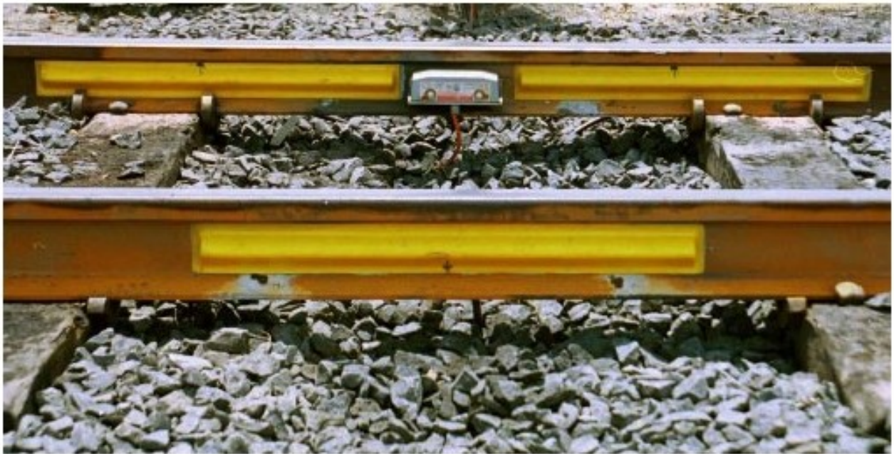
Meridian Engineers Model ME-AS41 Weighing Transducers
