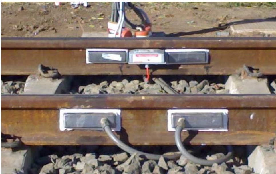
(b) Low speed TRACK-WEIGH 1A system (ME-AS60-A transducers)
