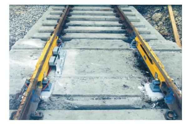
Weighing Transducers, Mounting Clamps and Track Switches
