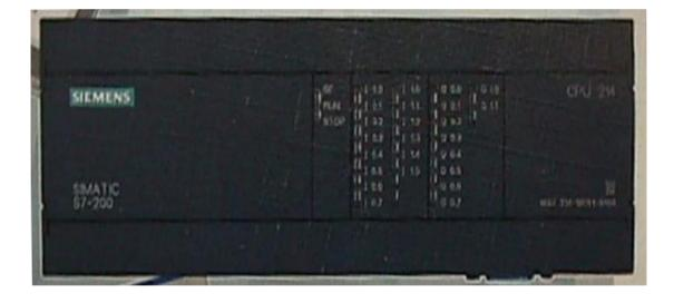
Seimens Model S7-200PLC Programmable Logic Controller
