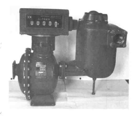
Brooks B-40 DB Meter, Strainer, and VR 7887 Indicator
