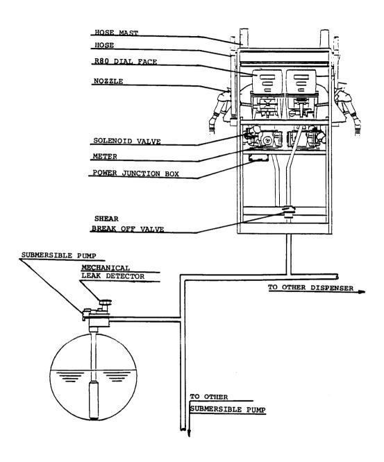
Typical Submersible Turbine Pump Hydraulic System
