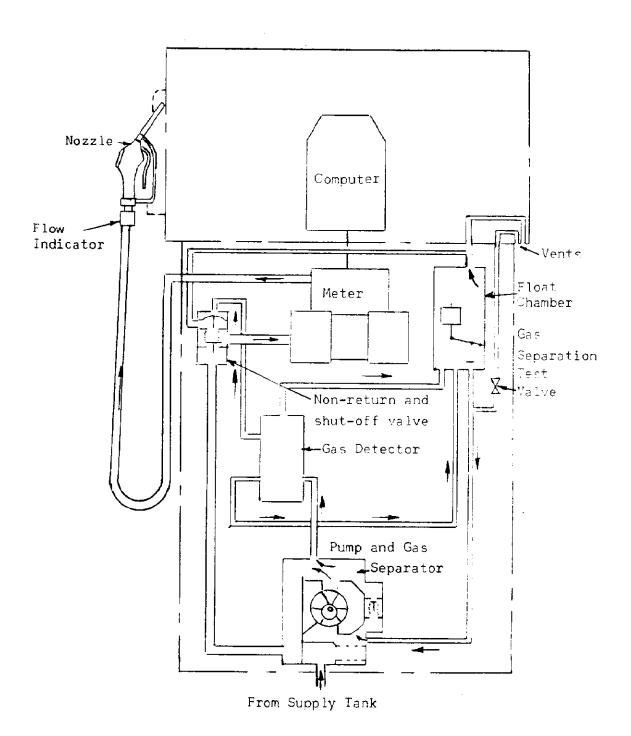
Hydraulic Diagram of Model ECC1D
