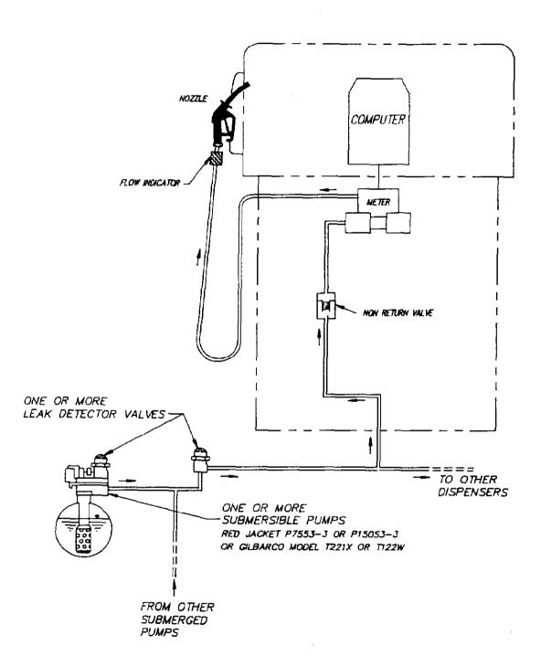
Typical System With a Submersible Turbine Pump
