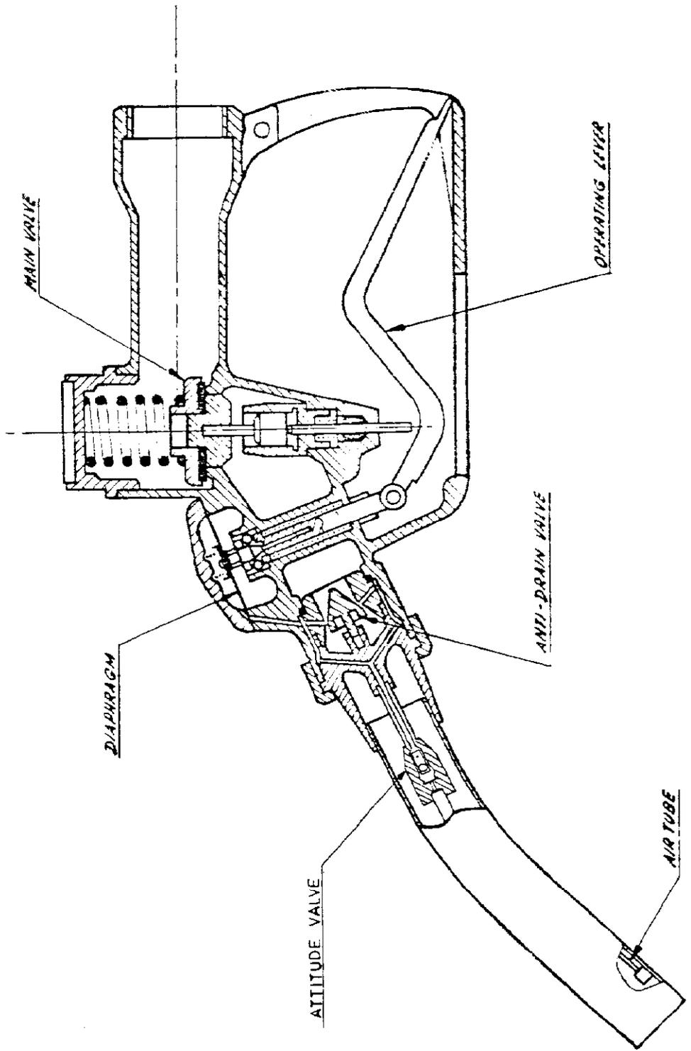
OPW IAS Automatic Hose Nozzle - Schematic Diagram
