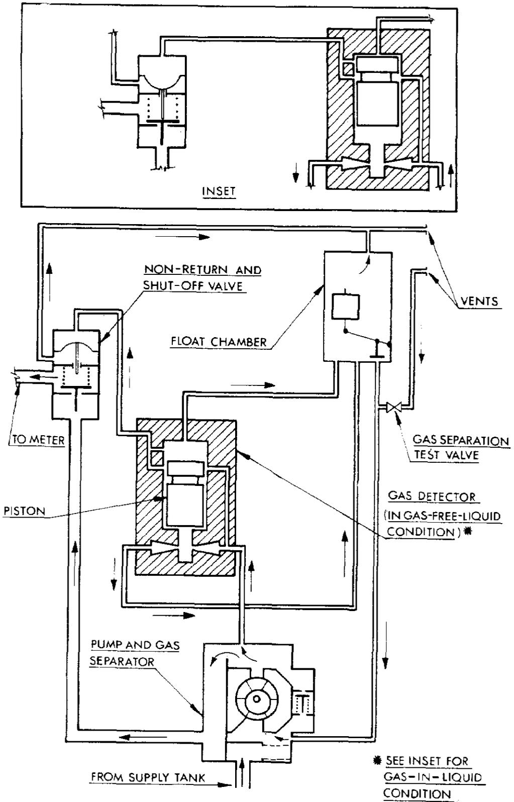
Wayne Gas-detector System - Hydraulic Diagram
