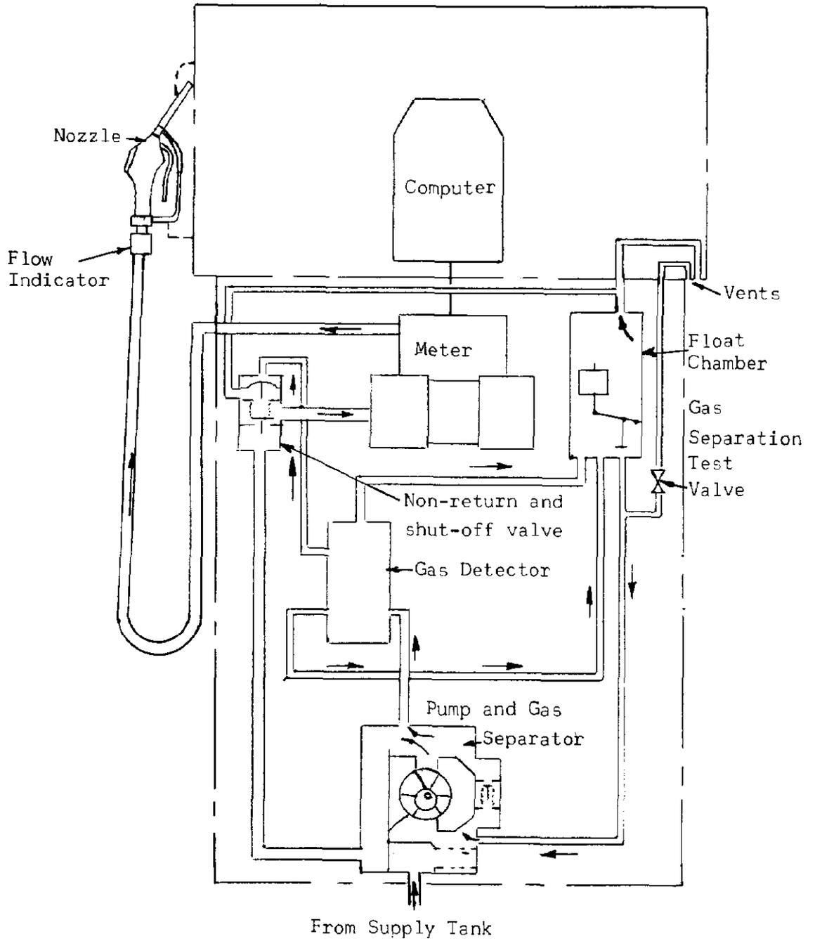
Hydraulic Diagram Model ECC1D, ECC1H and ECC1DH
