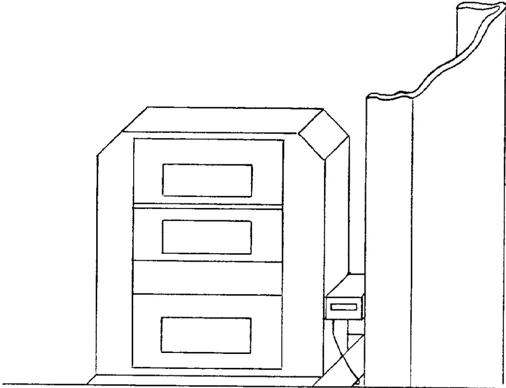
Electro-mechanical Totaliser Mounted on the Side Support of the Driveway Flowmeter Viewed through a hole in the Dial Plate
