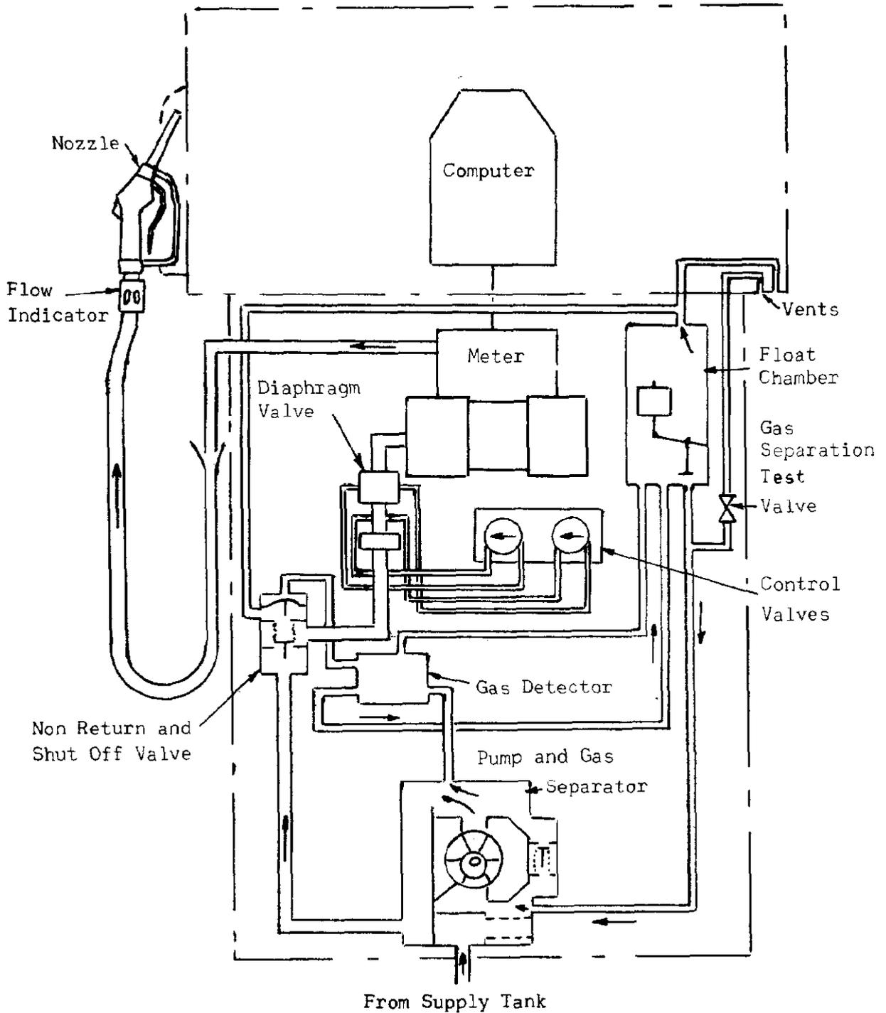
Hydraulic Diagram Model EDC1D, EDC1H and EDC1DH
