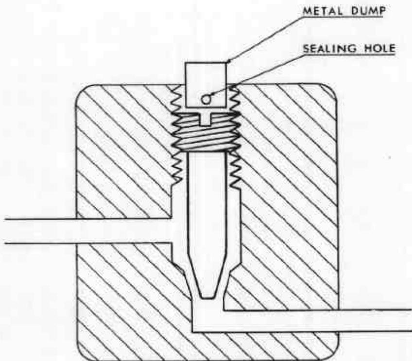
Gas-separator Test Valve — Schematic Diagram
