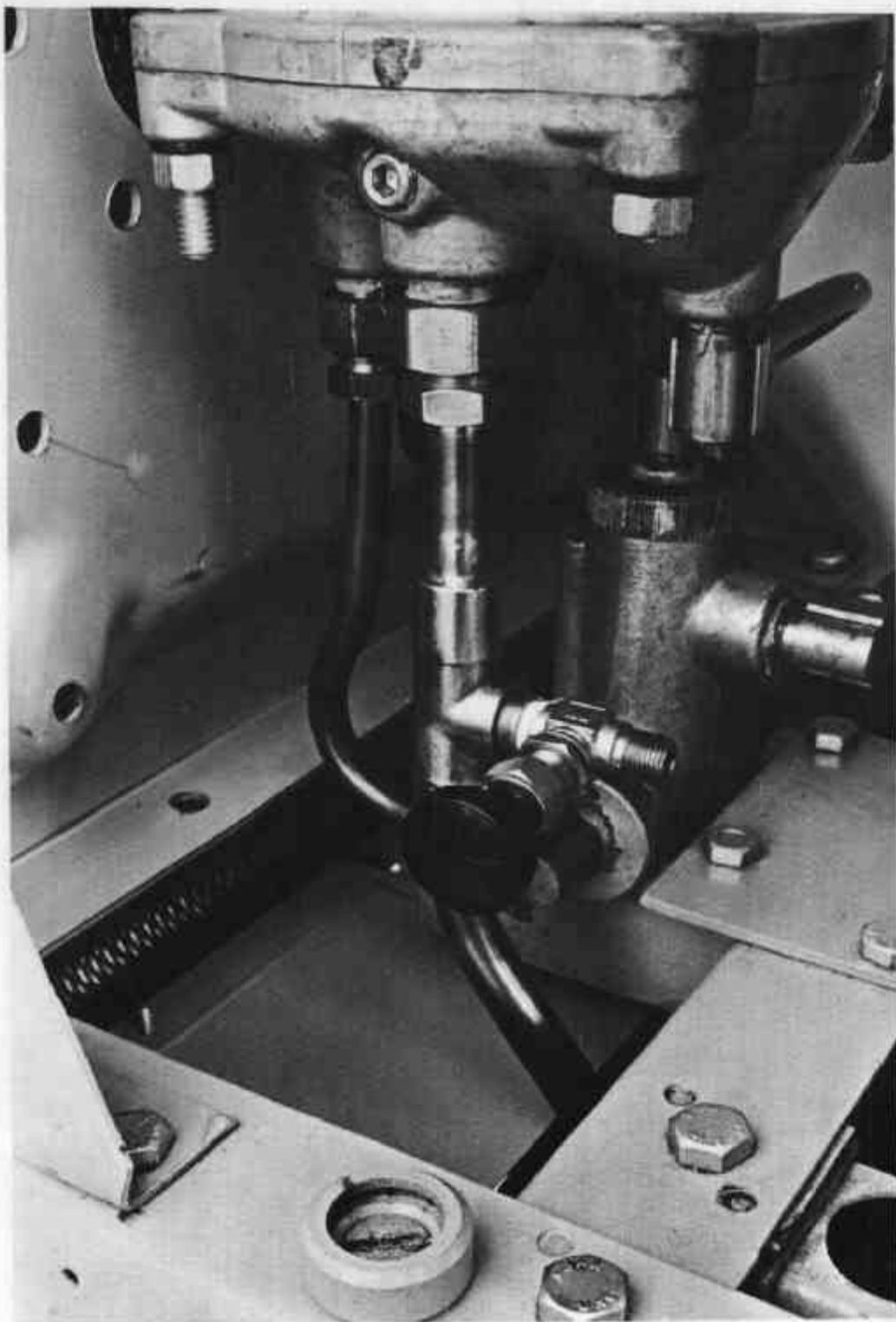
Gas-separation Test Valve
