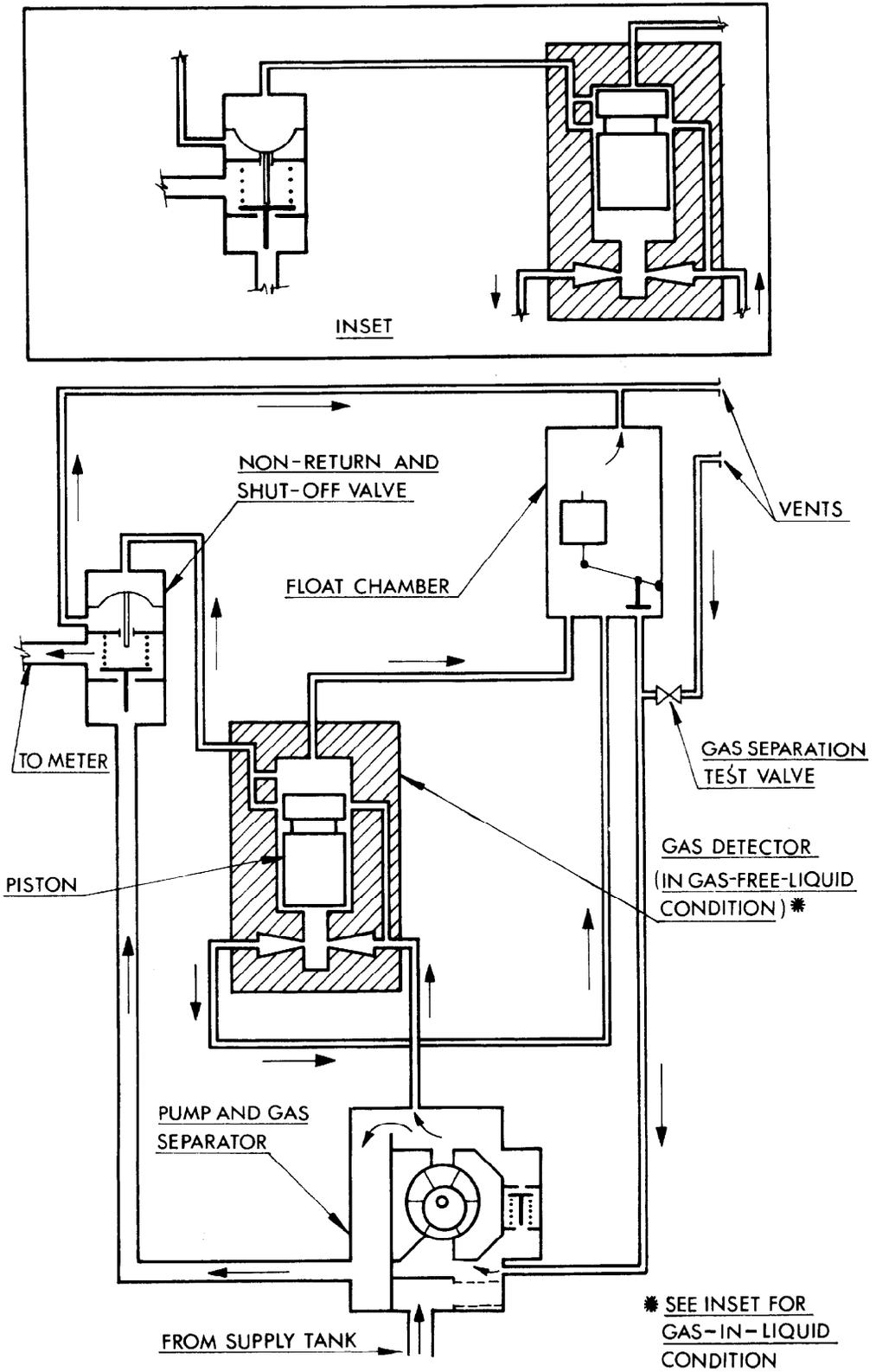
Wayne Gas Detector System - Hydraulic Diagram
