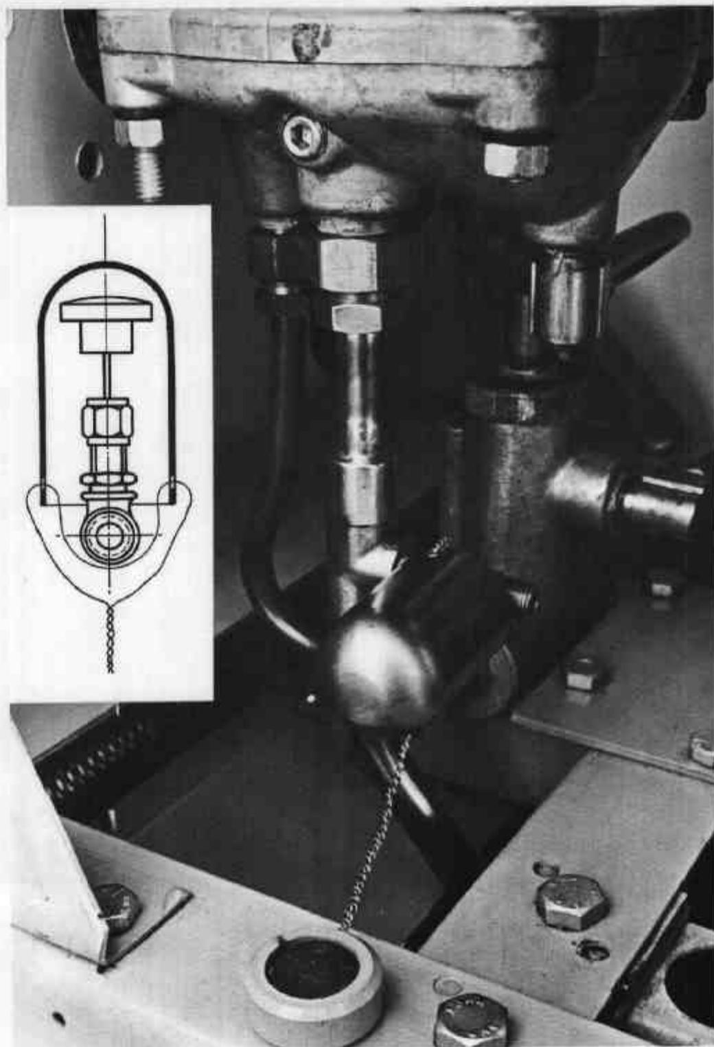
Gas-separation Test Valve — Method of Sealing (see inset)
