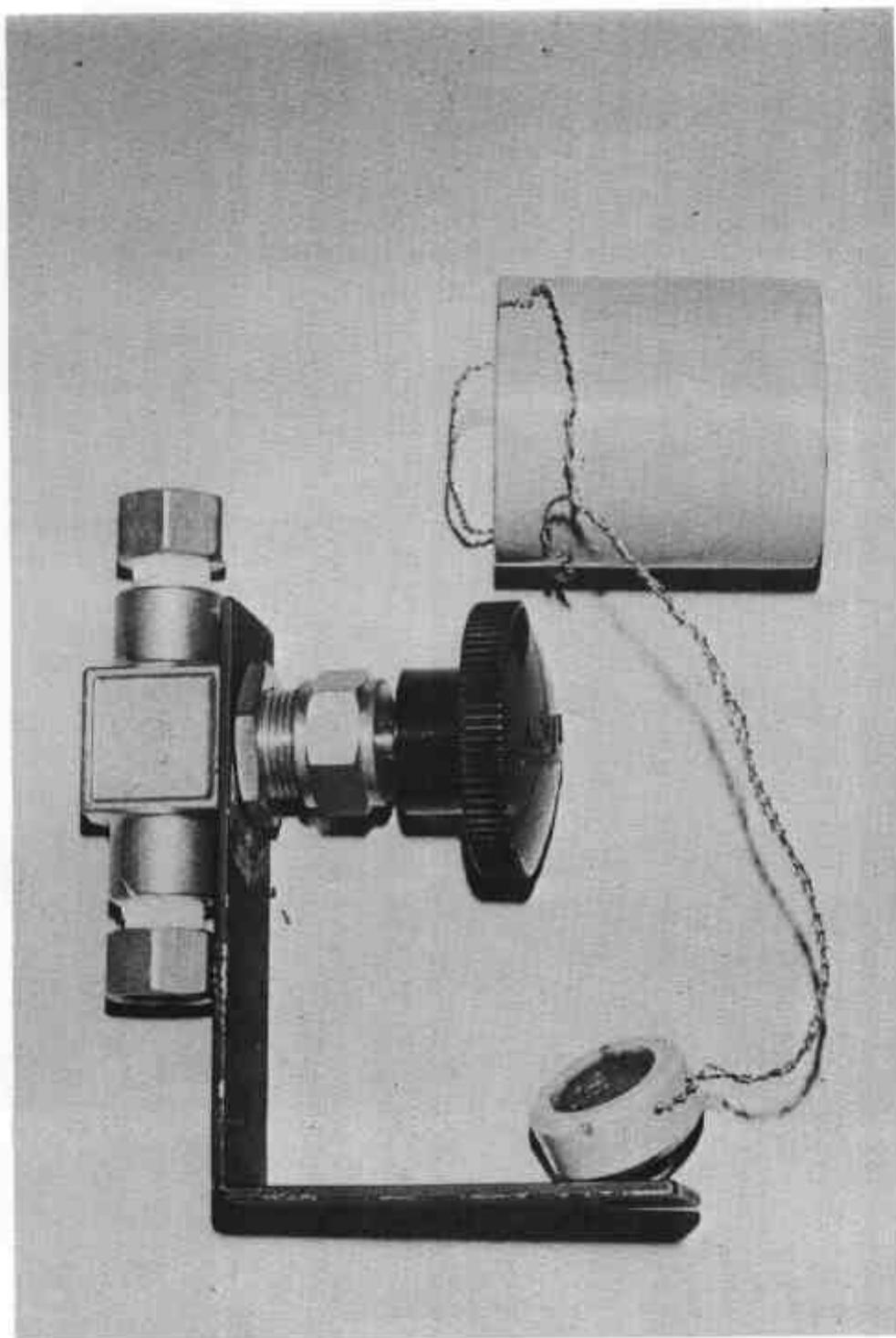
Gas-separation Test Valve and Sealing Cap
