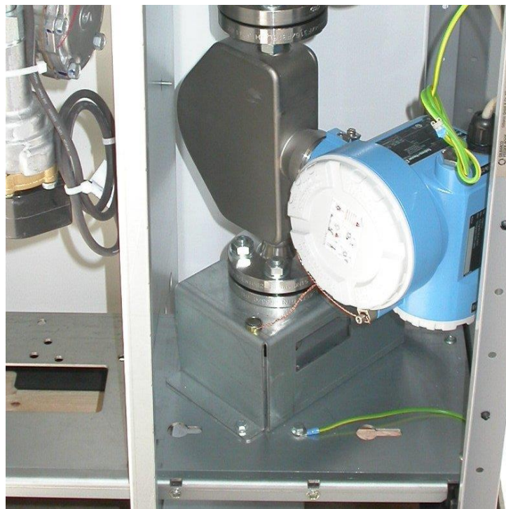
Typical Sealing of Coriolis Meter Calibration Access (Variant 13)
