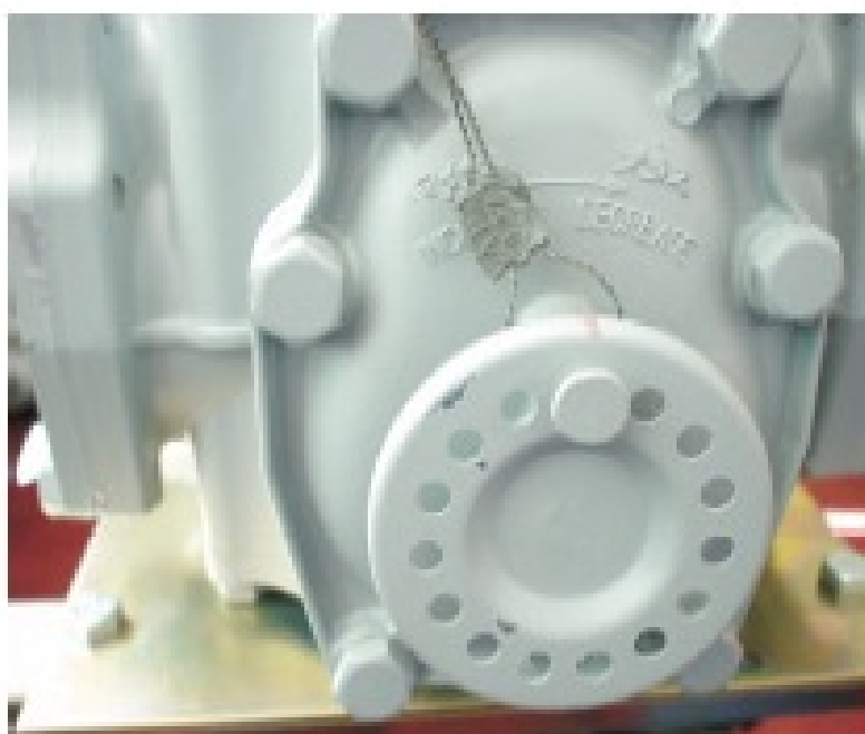
A Typical Sealing Method – Tatsuno Non-LPG Meter – The Pattern
