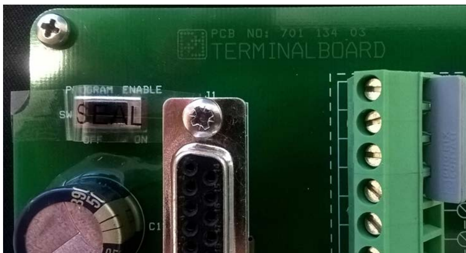
Typical Sealing of 'cal/measure' Switch for the Flow Sensor Electronics Module
