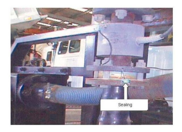
Turbo Messtechnik Model KF-G Flowmeter Including Sealing Method
