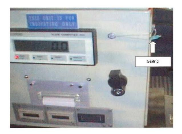
Sealing Method for Contrec Model 405D Calculator/Indicator
