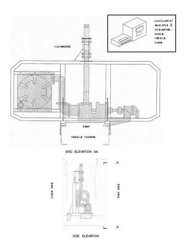
Typical Turbo Messtechnik Model KF-G Flowmetering System When Fitted to an Articulated Vehicle
