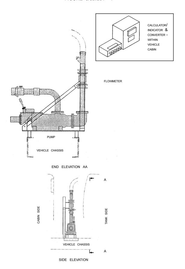
Typical Turbo Messtechnik Model KF-G Flowmetering System When Fitted to a Rigid Vehicle
